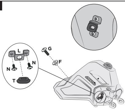
**Apply the two brackets (L) with the screws (N) and insert the original rubbers (T). Insert the screw (G) and the bushing (F).**
