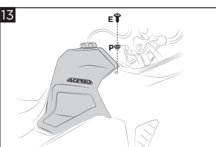
**Use the screws (E) and bushings (P) to fix the spoilers on both sides.**
