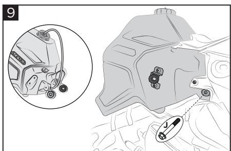
**Place the tank on the motorcycle and fix it using the screws (J) on both sides.**
