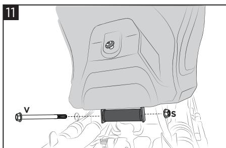
**Insert the screw (V) into the appropriate seat screw with the nut (S).**
