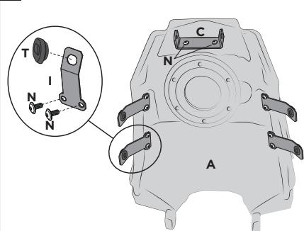
**Apply the four brackets (I) with the screws (N) and insert the original rubbers (T). Apply the bracket (C) using the screws (N) on the Acerbis fuel tank (A).**
