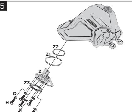
**Insert the pump (Z) and the gasket (Z1) using the screws (H) and washers (O).**
