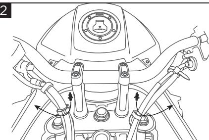
**Unhook the original pins from the carter, then remove the original tank.**
