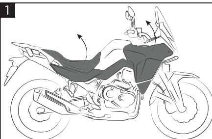
**Remove the original seat and radiator shrouds.**
