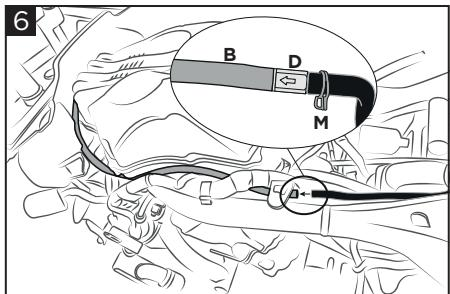
**Pull the hose (B) through as shown in figure and connect it to the carbon canister gas' original hose using the valve (D) and the clips (M).**
