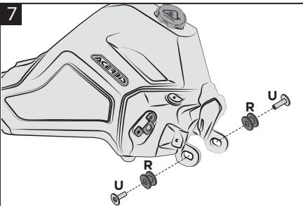
**Insert the rubbers (R) (after dismantling them from the original tank) and the bushings (U) before connecting the utilities.**
