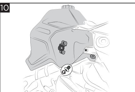
**Secure using the original screws (Q) on both sides.**
